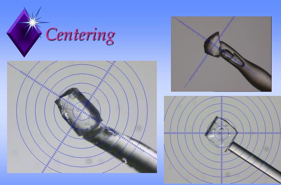
Sometimes the cross hairs do not represent the center of the x-ray beam and so rotation of the crystal by 180 degrees is done to facilitate alignment
