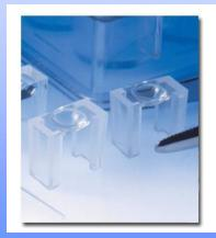
Plate Crystallizations, Hanging Drop Cover Slip Drop Grease Drop Contains Compound  $H_2O$  $H_2O$ Solvent A Over time the drop loses Solvent A to the lower reservoir and compound crystallizes Solvent A = Organic, water soluble solvent, Alcohols,  $CH_2Cl_2$
