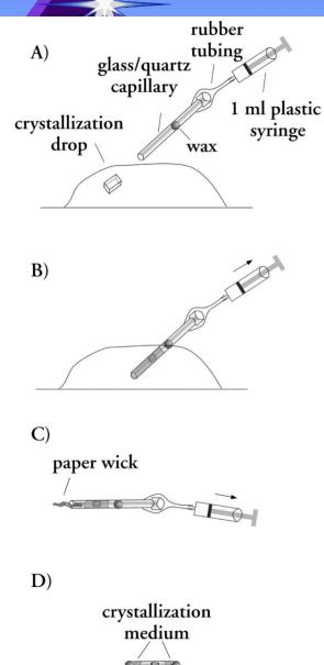
A) Assemble capillary, syringe and rubber tubing.
